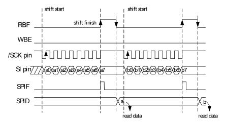
Fig. 16. Receive Mode (8-bit, 1 word)
